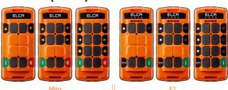
MINI+ (Plus) is the new compact pushbutton (200 g) that extends the range of model MINI. Configurations with 4-6-8 commands, clearly indicated; ergonomic shape with easy use with protection gloves, too. The electronic E1 can be supplied with single or two speed pushbuttons, category 3 PL d EN ISO 13849-1 stop function; 4 data feedback programmable Led. Powered by Lithium battery; USB power supply; USB cable Elca-Clip (AA batteries also available optional, without recharging).
